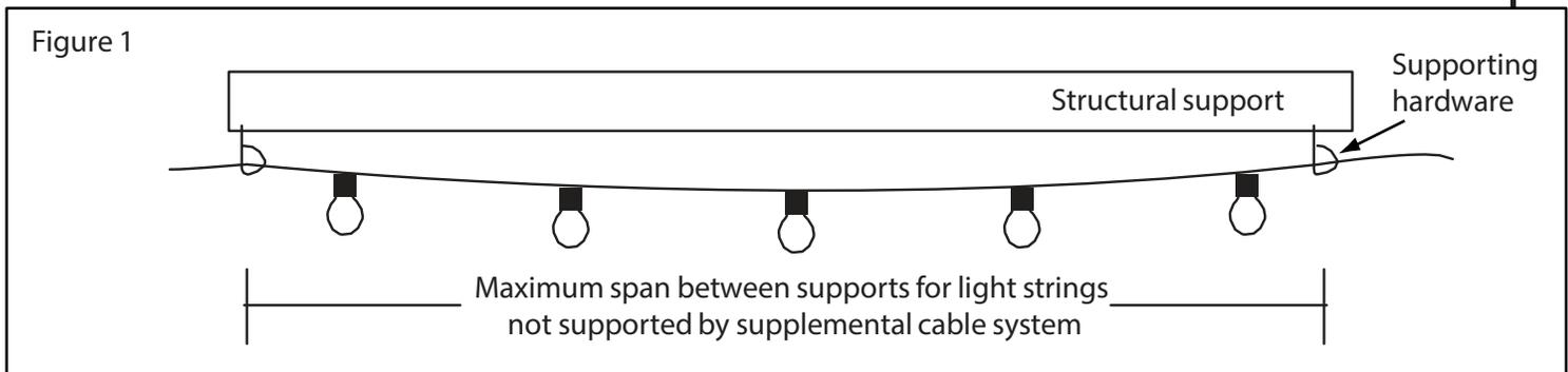
3. For spans exceeding the above, use properly rated [cable support system and cable ties](#) (both not provided) and follow local codes for suspended structures and loads.
